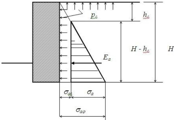
$$E_a = \frac{\gamma \cdot H^2}{2} \operatorname{tg}^2\left(45^\circ + \frac{\varphi}{2}\right) - 2cH \operatorname{tg}\left(45^\circ - \frac{\varphi}{2}\right) + \frac{2c^2}{\gamma}$$
